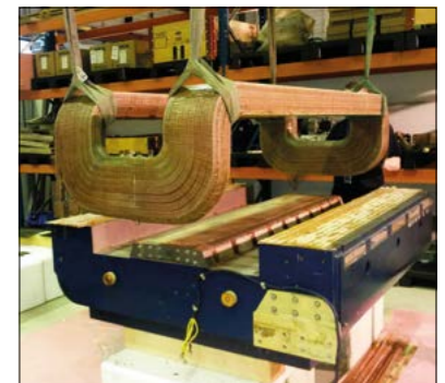
One of the 24 main bending magnets in the AD ring. Here the lower coil is being lifted out of the lower half of the magnet yoke. (Image credit: Tommy Eriksson.)
