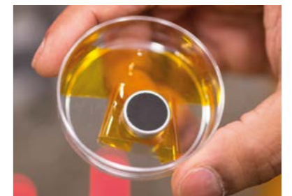
The dark carbon-nanotube-coated area of the new field-emission cathode. (Image credit: Fermilab.)
